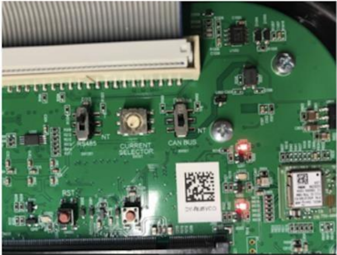
Close up RS485/ CAN bus switches
